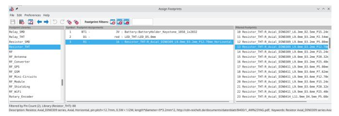
Many footprints are included with KiCad, so the footprint assignment tool offers several ways to filter out footprints that aren't relevant to the symbol in question.
