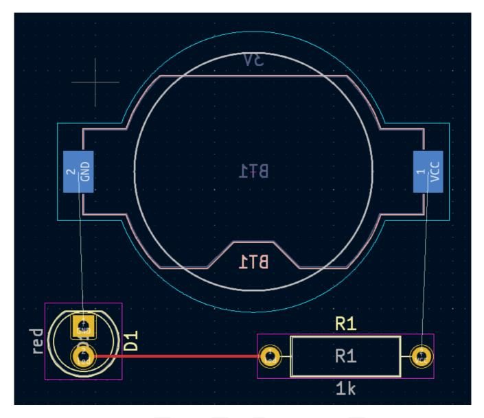
Now draw a trace between the GND pads of BT1 and D1, starting with the BT1 pad on the back of the board. Notice that the active layer automatically changed to B.Cu after clicking on the BT1 pad. Click on the D1 pad to finish the track.
