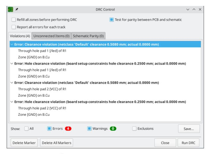
Close the DRC dialog, press B to refill the zone, and re-run DRC. Alternatively, check the *Refill all zones* before performing DRC checkbox and re-run DRC. All violations are fixed.
